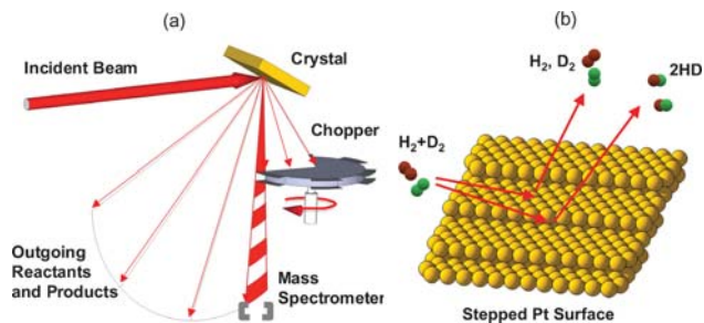
Fig. 5 (a) Schematic of molecular beam scattering studies. Detection of the scattered beam, desorbed reaction products or adsorbed species permits an understanding of the interaction between molecules and the surface. (b) High reactivity of H_2 – D_2 exchange revealed by molecular beam scattering.
